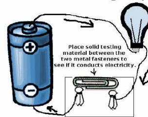
Solid Conductor Testing Setup
