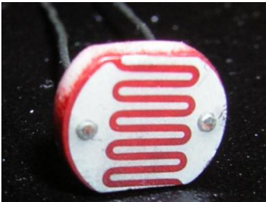
Figure 2: Cadmium Sulfide (CdS) photocells are used to sense vehicle roll rate and attitude
