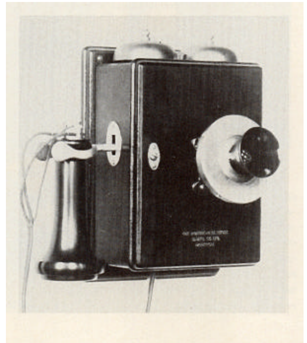
This 1904 wall telephone, installed at Ottawa without batteries or crank, depended on the common battery at the exchange and was less than one-half the size of earlier wall sets. Photo courtesy of Bell Canada Telephone Historical Collection.
