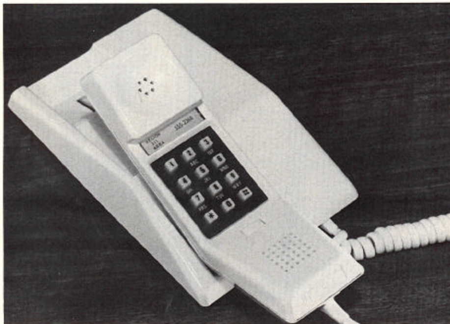
Le Contempra telephone, 1968, a Canadian design with mouthpiece, ear-phone and dial or Touch-Tone service integrated in handset. Photo courtesy of Bell Canada Telephone Historical Collection.
