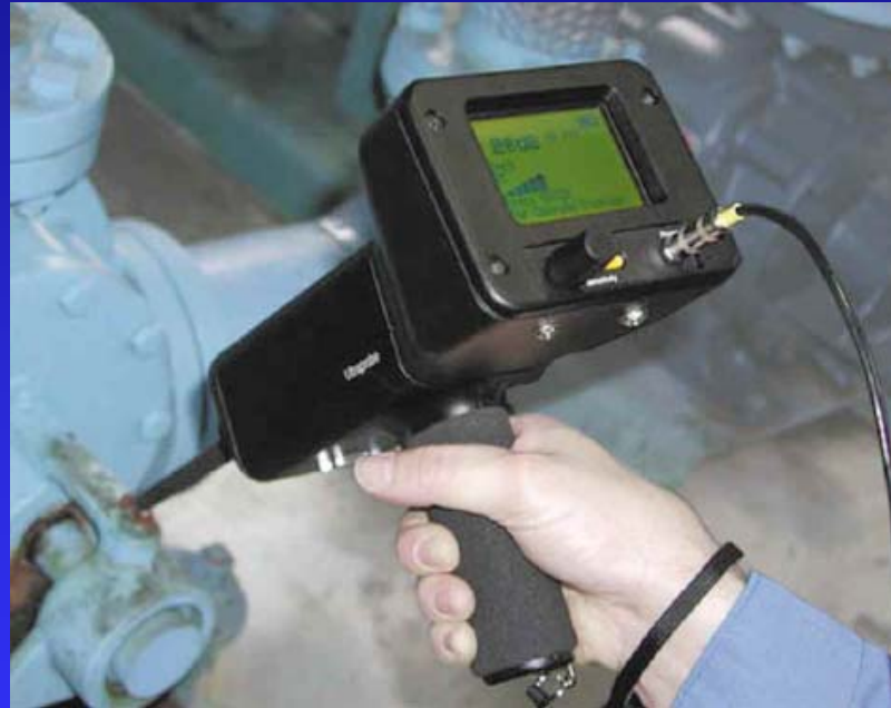
Ultrasonic detector Ultraprobe 10000 Digital Ultrasonic Inspection System, display panel and data views (Courtesy of UE Systems).
