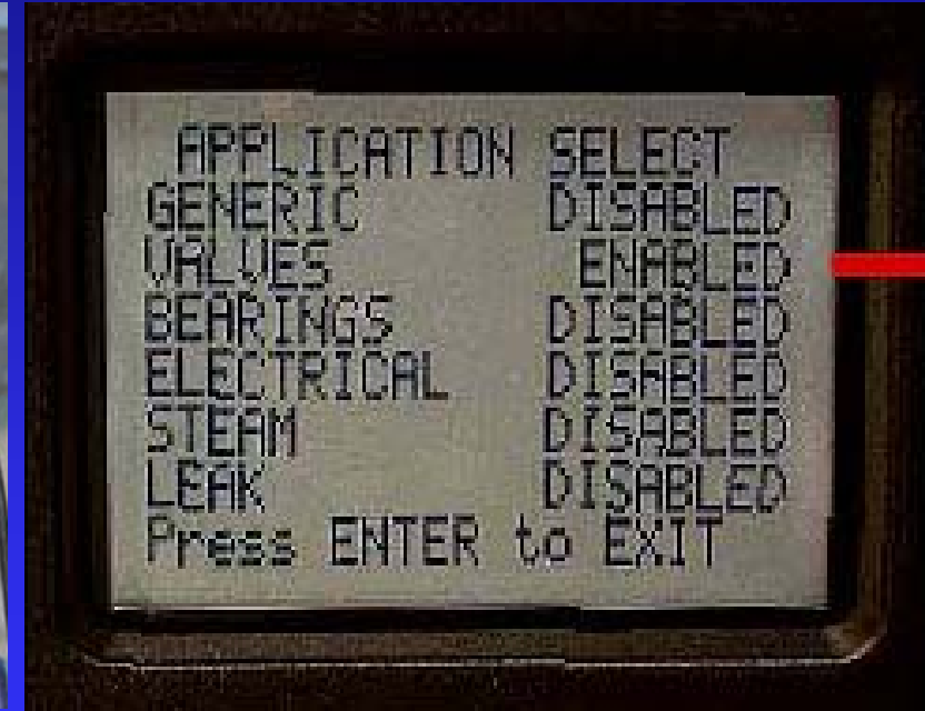
Ultrasonic detector Ultraprobe 10000 Digital Ultrasonic Inspection System, display panel and data views (Courtesy of UE Systems).
