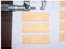
3 x 1 x 0.05" Ni/Au metallized Diamond/Al substrate
