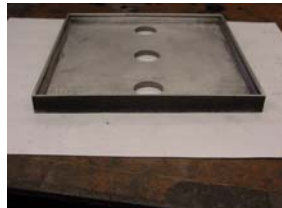
6 x 6 x 0.5" Diamond/Al enclosure With through holes
