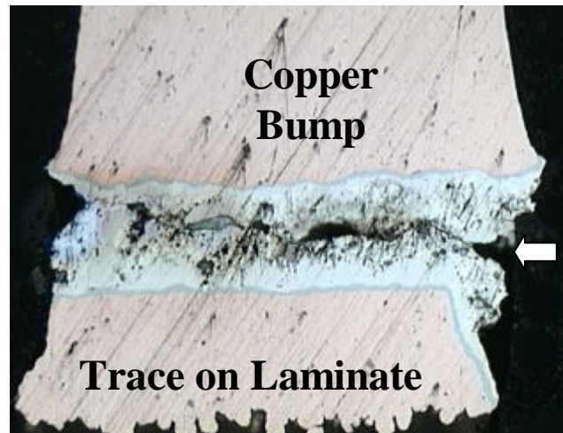
Figure 6. Typical Flip Chip Failure Cross-Section – Separation Within Solder.
