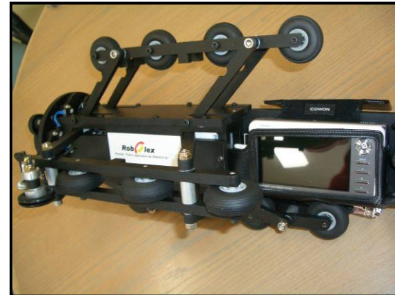
Duct camera system 'Robolex'™
