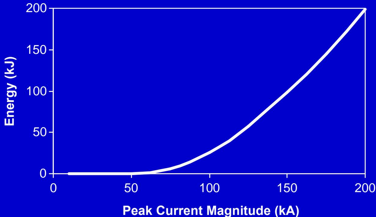
Stroke to a tower - Footing resistance:  $R_0 = 50 \Omega$ ;  $\rho = 200 \Omega.m$
