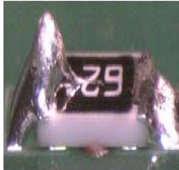
Icicing of SMD using No-clean ROLO Flux
