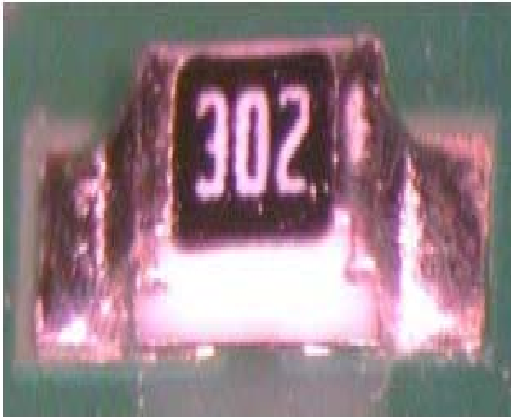
Well soldered SMD bottom-side
