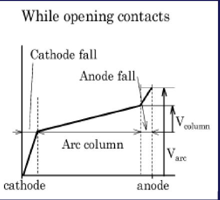
Ref: Voltage-Current Characteristics of Breaking Arc at Constant Opening Speed in the Air, Sekikawa et all, IEEE Transactions on Components & Packaging Technologies, Vol. 27, No. 1, March 2004
