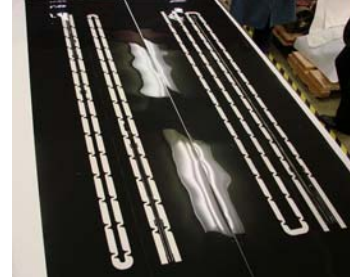
Fig. 5. Artwork of LQ layer 1 and layer 2 traces
