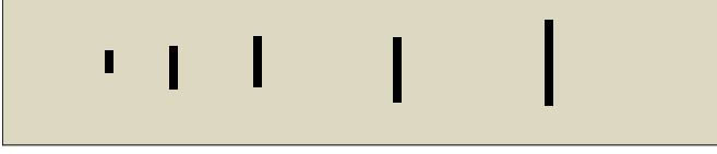
Fig. 2. A sketch of Sample 2 with the 5 artificial defects made by laser cutting. The tape width is 10 mm, the length is 65 mm.
