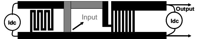
Fig. 11. Possible configuration of an SSPD integrated with a pulse amplifier. The black lines represent superconducting wires, the gray ones resistive wires.
