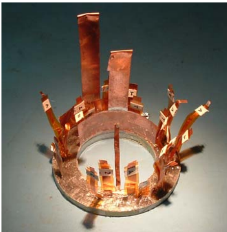
Fig. 5 Small pancake coil using first length of 10 m of 344 superconductors (see Table 1), with current leads and voltage taps (wide and narrow Cu foils) and centrally located heater, one full turn, for stability testing in liquid He.
