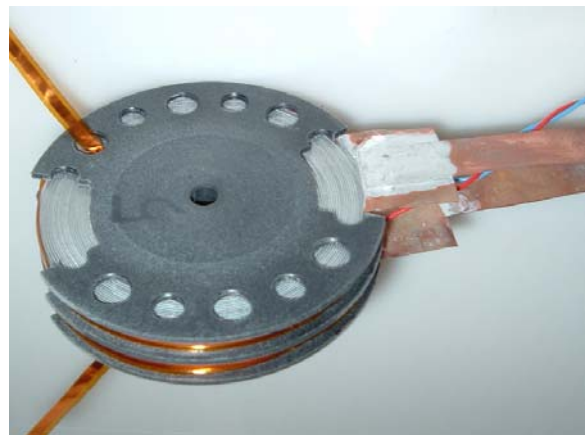
Fig. 3. Double pancake coil wound on polymer pre-form. Slots were machined for current lead access and pancake-to-pancake connection.
