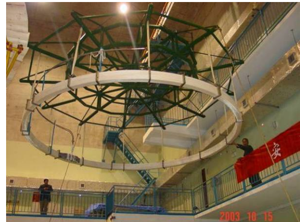
Fig. 3. One of the PF coils of the EAST machine.
