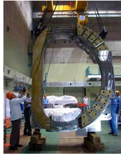
Fig. 2. One of the TF coils of the EAST machine
