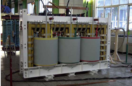
Fig. 17. Overview of the 630 kVA 10.5 kV/0.4 kV transformer
