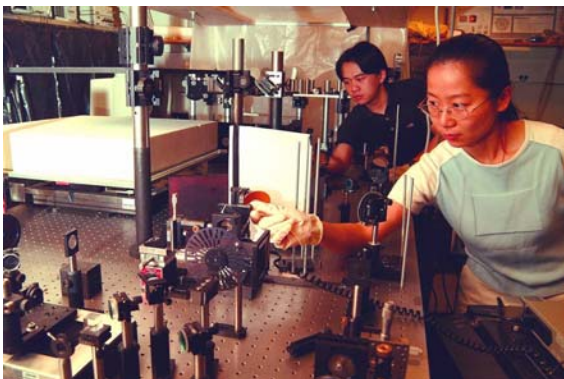
Ms. Zhong and Mr. Xie use THz wave to measure the defects in the space shuttle insulation foams.
