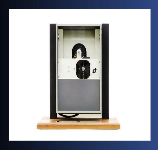
1962 – IBM 1311 Disk Drive was the first removable data storage device.
